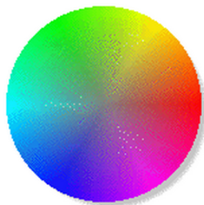
Figure 3.5: color wheel - A sample absorbs visible light of color of the specific wavelength and reflects the rest, in appears the complementary color of light. Find the color that is absorbed, then move directly across the wheel to the other side to get the complement.
