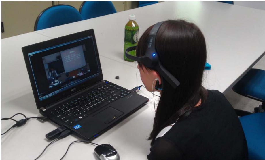
Figure 4. The experimental scene of a learner who simultaneously wore a Mindset earphone and an emWave stress detector to assess sustained attention and emotion while performing an autonomous online learning by video lecture
