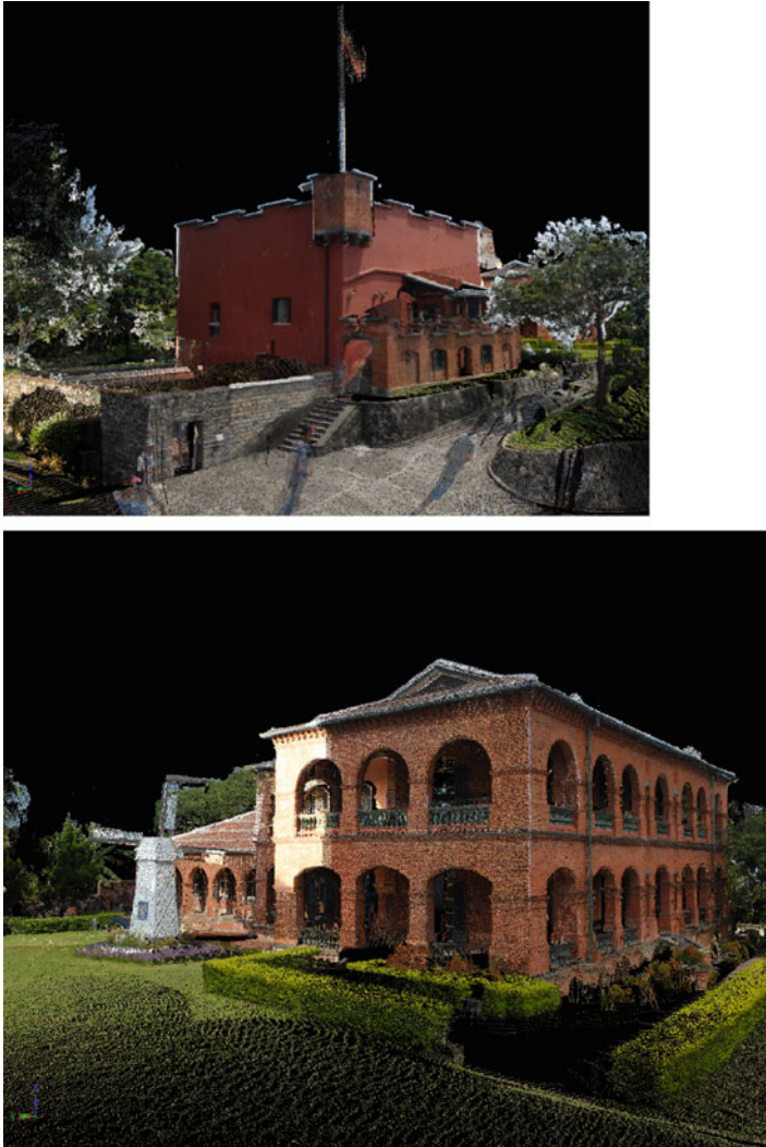
Fig. 8.5 The scanned model of Fort Antonio ( top ) and former British Consular Residence ( bottom ). The models are textured with color extracted from the imagery acquired by the digital camera mounted on the scanner
