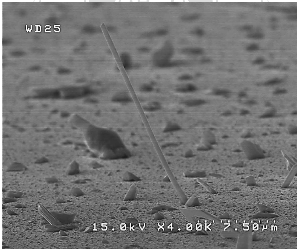
Figure 3.16 Side view SEM image of \text{Bi}_{0.5}\text{Sb}_{1.5}\text{Te}_3 film after annealing at 350\text{ }^\circ\text{C} for 21 days.
