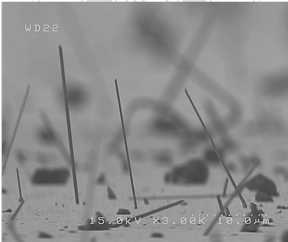
Figure 3.18 Side view SEM image of Bi 1.5 Sb 1.0 Te 3 film after annealing at 490 °C for 5 days.
