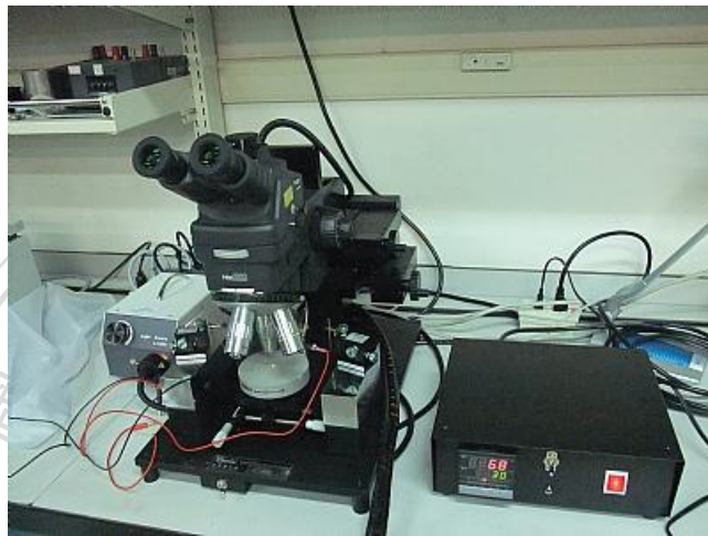
Figure 4.1 Set up of probe station with micropositioner for manipulating nanowire.
