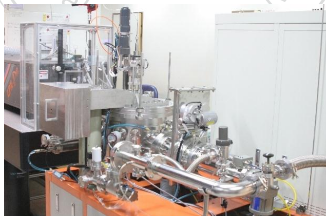
Figure 3.3 Pulsed laser deposition system for nanoparticles and thin film fabrication.
