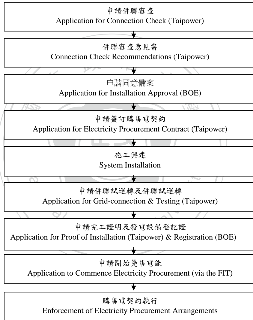
Figure 2: New Administrative Procedures Based on the Draft Amendments to the Renewable Energy Installations Approval Process 再生能源發電設備認定辦法修正草案總說明
